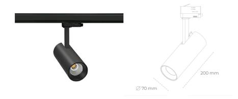
COB 4000 [K] HI EFFICIENT Light colour CRI 90 Led chip flux 2260 [lm] Luminous flux 1808 [lm] System power 14 [W] Luminaire Efficiency 129 [lm/W] Beam angle 15° Controller ON/OFF MacAdam 3 SDCM
