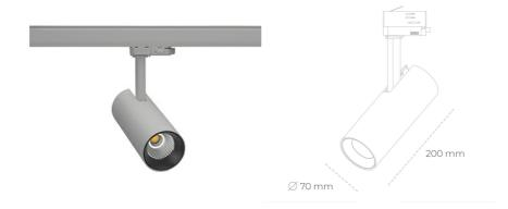
COB 2500 [K] BREAD Light colour CRI 2340 [lm] Led chip flux Luminous flux 1872 [lm] System power 19 [W] Luminaire Efficiency 99 [lm/W] Beam angle 60° Controller ON/OFF MacAdam 3 SDCM
