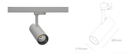
COB 2500 [K] BREAD Light colour CRI 1195 [lm] Led chip flux Luminous flux 956 [lm] System power 10 [W] Luminaire Efficiency 96 [lm/W] Beam angle 38° Controller ON/OFF MacAdam 3 SDCM
