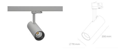
COB 2000 [K] MEAT PINK Light colour CRI 895 [lm] Led chip flux Luminous flux 716 [lm] System power 10 [W] Luminaire Efficiency 72 [Im/W] Beam angle 38° Controller ON/OFF MacAdam 3 SDCM
