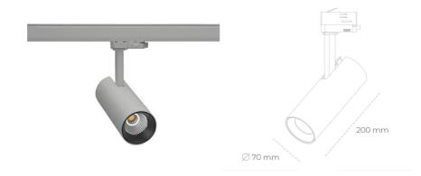
COB 2000 [K] MEAT PINK Light colour CRI Led chip flux 1253 [lm] Luminous flux 1002 [lm] System power 14 [W] Luminaire Efficiency 72 [Im/W] Beam angle 15° Controller ON/OFF MacAdam 3 SDCM
