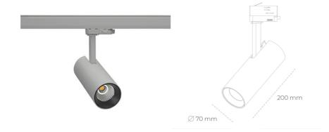
COB 3000 [K] CRI97 Light colour CRI 2199 [lm] Led chip flux Luminous flux 1759 [lm] System power 19 [W] Luminaire Efficiency 93 [lm/W] Beam angle 24° Controller ON/OFF MacAdam 3 SDCM
