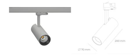
COB 5700 [K] SPECIAL Light colour CRI Led chip flux 1820 [lm] Luminous flux 1456 [lm] System power 14 [W] Luminaire Efficiency 104 [lm/W] Beam angle 60° Controller ON/OFF
