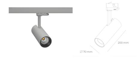
COB 5700 [K] SPECIAL Light colour CRI 2788 [lm] Led chip flux Luminous flux 2230 [lm] System power 21 [W] Luminaire Efficiency 106 [lm/W] Beam angle 38° Controller ON/OFF MacAdam 3 SDCM
