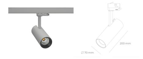
COB 5700 [K] SPECIAL Light colour CRI Led chip flux 2551 [lm] Luminous flux 2040 [lm] System power 19 [W] Luminaire Efficiency 107 [lm/W] Beam angle 38° Controller ON/OFF MacAdam 3 SDCM
