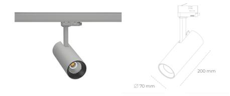
COB 5700 [K] SPECIAL Light colour CRI 1820 [lm] Led chip flux Luminous flux 1456 [lm] System power 14 [W] Luminaire Efficiency 104 [lm/W] Beam angle 15° Controller ON/OFF
