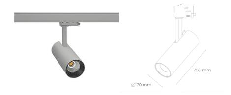
COB 4200 [K] MEAT WHITE Light colour CRI 90 Led chip flux 1976 [lm] Luminous flux 1580 [lm] System power 19 [W] Luminaire Efficiency 83 [lm/W] Beam angle 38° Controller ON/OFF MacAdam 3 SDCM
