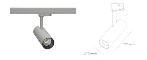
COB 4200 [K] MEAT WHITE Light colour CRI 90 Led chip flux 1412 [lm] Luminous flux 1129 [lm] System power 14 [W] Luminaire Efficiency 81 [lm/W] Beam angle 24° Controller ON/OFF MacAdam 3 SDCM
