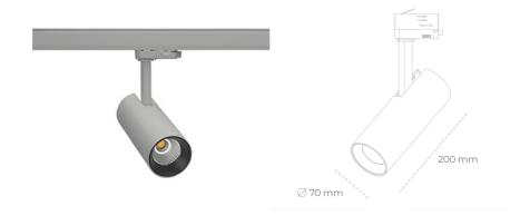
COB 4200 [K] MEAT WHITE Light colour CRI 90 Led chip flux 2159 [lm] Luminous flux 1727 [lm] System power 21 [W] Luminaire Efficiency 82 [lm/W] Beam angle 15° Controller ON/OFF MacAdam 3 SDCM
