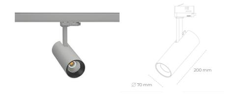
COB 4200 [K] MEAT WHITE Light colour CRI 90 Led chip flux 1976 [lm] Luminous flux 1580 [lm] System power 19 [W] Luminaire Efficiency 83 [lm/W] Beam angle 15° Controller ON/OFF MacAdam 3 SDCM
