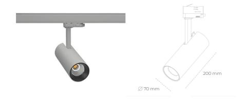
COB 3500 [K] HI EFFICIENT Light colour CRI 90 Led chip flux 3341 [lm] Luminous flux 2672 [lm] System power 21 [W] Luminaire Efficiency 127 [lm/W] Beam angle 38° Controller ON/OFF MacAdam 3 SDCM
