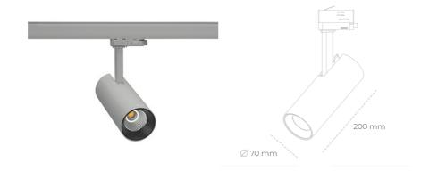
COB 3500 [K] HI EFFICIENT Light colour CRI 90 Led chip flux 3341 [lm] Luminous flux 2672 [lm] System power 21 [W] Luminaire Efficiency 127 [lm/W] Beam angle 24° Controller ON/OFF MacAdam 3 SDCM
