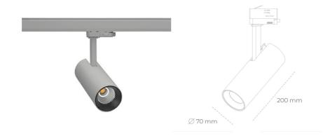
COB 3000 [K] HI EFFICIENT Light colour CRI 90 Led chip flux 3184 [lm] Luminous flux 2547 [lm] System power 19 [W] Luminaire Efficiency 134 [lm/W] Beam angle 24° Controller ON/OFF MacAdam 3 SDCM
