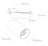
COB 2500 [K] BREAD Light colour CRI 3169 [lm] Led chip flux Luminous flux 2535 [lm] System power 27 [W] Luminaire Efficiency 94 [lm/W] Beam angle 30° Controller ON/OFF
