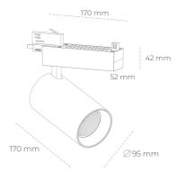
COB 2500 [K] BREAD Light colour CRI Led chip flux 1195 [lm] Luminous flux 956 [lm] System power 10 [W] Luminaire Efficiency 96 [lm/W] Beam angle 15° Controller ON/OFF
