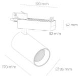
LED COB Light colour 4000 [K] | CRI 90 Led chip flux 1691 [lm] Luminous flux 1352 [lm] System power 14 [W] Luminaire Efficiency 97 [lm/W] 45° Beam angle Controller ON/OFF
