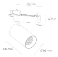
COB 5700 [K] SPECIAL Light colour CRI 3255 [lm] Led chip flux Luminous flux 2604 [lm] System power 25 [W] Luminaire Efficiency 104 [lm/W] Beam angle 30° Controller ON/OFF
