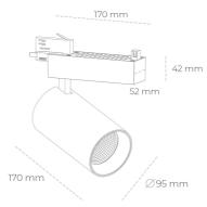
COB 4200 [K] MEAT WHITE Light colour CRI 90 Led chip flux 1412 [lm] Luminous flux 1129 [lm] System power 14 [W] Luminaire Efficiency 81 [lm/W] Beam angle 15° Controller ON/OFF MacAdam
