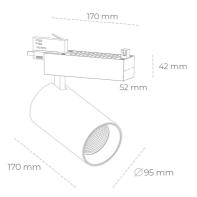
COB 4000 [K] HI EFFICIENT Light colour CRI 90 Led chip flux 4964 [lm] Luminous flux 3971 [lm] System power 31 [W] Luminaire Efficiency 128 [lm/W] Beam angle 30° Controller ON/OFF MacAdam 3 SDCM
