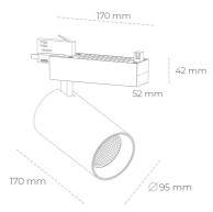
COB 4000 [K] HI EFFICIENT Light colour CRI 90 Led chip flux 2260 [lm] Luminous flux 1808 [lm] System power 14 [W] Luminaire Efficiency 129 [lm/W] Beam angle 15° Controller ON/OFF MacAdam 3 SDCM
