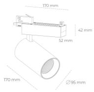
COB 3500 [K] HI EFFICIENT Light colour CRI 90 Led chip flux 3341 [lm] Luminous flux 2672 [lm] System power 21 [W] Luminaire Efficiency 127 [lm/W] Beam angle 45° Controller ON/OFF MacAdam 3 SDCM
