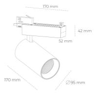
COB 3500 [K] HI EFFICIENT Light colour CRI 90 Led chip flux 1571 [lm] Luminous flux 1256 [lm] System power 10 [W] Luminaire Efficiency 126 [lm/W] Beam angle 30° Controller ON/OFF MacAdam 3 SDCM
