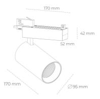
COB 2000 [K] MEAT PINK Light colour CRI Led chip flux 1741 [lm] Luminous flux 1392 [lm] System power 19 [W] Luminaire Efficiency 73 [Im/W] Beam angle 15° Controller ON/OFF MacAdam 3 SDCM
