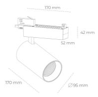
COB 4000 [K] PREMIUM WHITE Light colour CRI 90 Led chip flux 4097 [lm] Luminous flux 3277 [lm] System power 31 [W] Luminaire Efficiency 106 [lm/W] Beam angle 45° Controller ON/OFF MacAdam 3 SDCM
