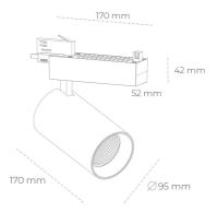
COB 5700 [K] SPECIAL Light colour CRI Led chip flux 2551 [lm] Luminous flux 2040 [lm] System power 19 [W] Luminaire Efficiency 107 [lm/W] Beam angle 15° Controller ON/OFF MacAdam 3 SDCM
