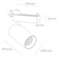
COB 4200 [K] MEAT WHITE Light colour CRI 90 Led chip flux 1976 [lm] Luminous flux 1580 [lm] System power 19 [W] Luminaire Efficiency 83 [lm/W] Beam angle 15° Controller ON/OFF MacAdam 3 SDCM
