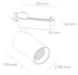
Track mounted LED spotlight. Aluminium housing. Ceiling base
