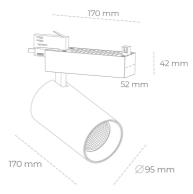
COB 4000 [K] HI EFFICIENT Light colour CRI 90 Led chip flux 4964 [lm] Luminous flux 3971 [lm] System power 31 [W] Luminaire Efficiency 128 [lm/W] Beam angle 15° Controller ON/OFF MacAdam 3 SDCM
