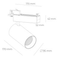
COB 3500 [K] HI EFFICIENT Light colour CRI 90 Led chip flux 3624 [lm] Luminous flux 2899 [lm] System power 23 [W] Luminaire Efficiency 126 [lm/W] Beam angle 45° Controller ON/OFF MacAdam 3 SDCM
