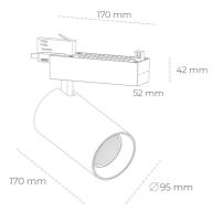
COB 3500 [K] HI EFFICIENT Light colour CRI 90 Led chip flux 3054 [lm] Luminous flux 2443 [lm] System power 19 [W] Luminaire Efficiency 129 [lm/W] Beam angle 45° Controller ON/OFF MacAdam 3 SDCM
