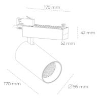
COB 3500 [K] HI EFFICIENT Light colour CRI 90 Led chip flux 3624 [lm] Luminous flux 2899 [lm] System power 23 [W] Luminaire Efficiency 126 [lm/W] Beam angle 30° Controller ON/OFF MacAdam 3 SDCM
