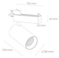
COB 3000 [K] HI EFFICIENT Light colour CRI 90 Led chip flux 3787 [lm] Luminous flux 3029 [lm] System power 23 [W] Luminaire Efficiency 132 [lm/W] Beam angle 45° Controller ON/OFF MacAdam 3 SDCM
