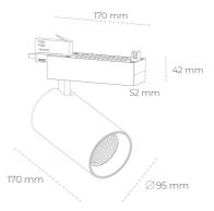
COB 3000 [K] HI EFFICIENT Light colour CRI 90 Led chip flux 3487 [lm] Luminous flux 2789 [lm] System power 21 [W] Luminaire Efficiency 133 [lm/W] Beam angle 45° Controller ON/OFF MacAdam 3 SDCM
