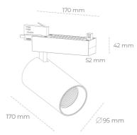
COB 3000 [K] HI EFFICIENT Light colour CRI 90 Led chip flux 2256 [lm] Luminous flux 1804 [lm] System power 14 [W] Luminaire Efficiency 129 [lm/W] Beam angle 30° Controller ON/OFF MacAdam 3 SDCM
