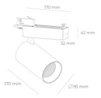
COB 2500 [K] BREAD Light colour CRI Led chip flux 1195 [lm] Luminous flux 956 [lm] System power 10 [W] Luminaire Efficiency 96 [lm/W] Beam angle 30° Controller ON/OFF MacAdam 3 SDCM
