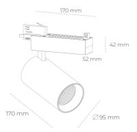
COB 2500 [K] BREAD Light colour CRI 2808 [lm] Led chip flux Luminous flux 2246 [lm] System power 23 [W] Luminaire Efficiency 98 [lm/W] Beam angle 15° Controller ON/OFF MacAdam 3 SDCM
