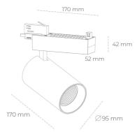
COB 2000 [K] MEAT PINK Light colour CRI 2349 [lm] Led chip flux Luminous flux 1879 [lm] System power 27 [W] Luminaire Efficiency 70 [lm/W] Beam angle 30° Controller ON/OFF MacAdam 3 SDCM
