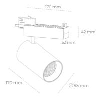
COB 2000 [K] MEAT PINK Light colour CRI Led chip flux 2181 [lm] Luminous flux 1744 [lm] System power 25 [W] Luminaire Efficiency 70 [lm/W] Beam angle 30° Controller ON/OFF MacAdam 3 SDCM
