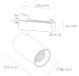
Light colour 2700 [K] | CRI 80 Led chip flux 2444 [lm] Luminous flux 1955 [lm] System power 21 [W] Luminaire Efficiency 93 [lm/W] 45° Beam angle Controller ON/OFF
