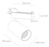
LED COB Light colour 2700 [K] | CRI 80 Led chip flux 3555 [lm] Luminous flux 2844 [lm] System power 31 [W] Luminaire Efficiency 92 [lm/W] 30° Beam angle Controller ON/OFF
