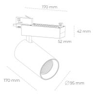
COB Light colour 2700 [K] | CRI Led chip flux 3233 [lm] Luminous flux 2586 [lm] System power 23 [W] Luminaire Efficiency 112 [lm/W] Beam angle 15° Controller ON/OFF MacAdam 3 SDCM
