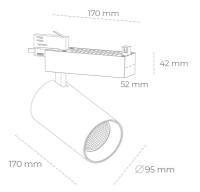
COB 3000 [K] CRI97 Light colour CRI Led chip flux 2601 [lm] Luminous flux 2080 [lm] System power 23 [W] Luminaire Efficiency 90 [lm/W] Beam angle 45° Controller ON/OFF MacAdam 3 SDCM
