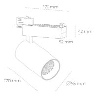
COB 3000 [K] CRI97 Light colour CRI Led chip flux 2402 [lm] Luminous flux 1921 [lm] System power 21 [W] Luminaire Efficiency 91 [lm/W] Beam angle 15° Controller ON/OFF MacAdam 3 SDCM
