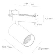
COB 4200 [K] MEAT WHITE Light colour CRI 90 Led chip flux 2159 [lm] Luminous flux 1727 [lm] System power 21 [W] Luminaire Efficiency 82 [lm/W] Beam angle 45° Controller ON/OFF MacAdam 3 SDCM
