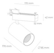
COB 4200 [K] MEAT WHITE Light colour CRI 90 Led chip flux 2695 [lm] Luminous flux 2156 [lm] System power 27 [W] Luminaire Efficiency 80 [lm/W] Beam angle 30° Controller ON/OFF MacAdam 3 SDCM
