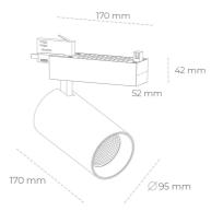
COB 4200 [K] MEAT WHITE Light colour CRI 90 Led chip flux 2159 [lm] Luminous flux 1727 [lm] System power 21 [W] Luminaire Efficiency 82 [lm/W] Beam angle 30° Controller ON/OFF MacAdam 3 SDCM
